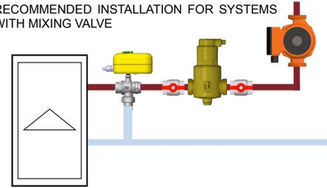
**⚠ Note!** To operate efficiently, the deaerator should always be installed in a horizontal pipe run, with the body upright.
