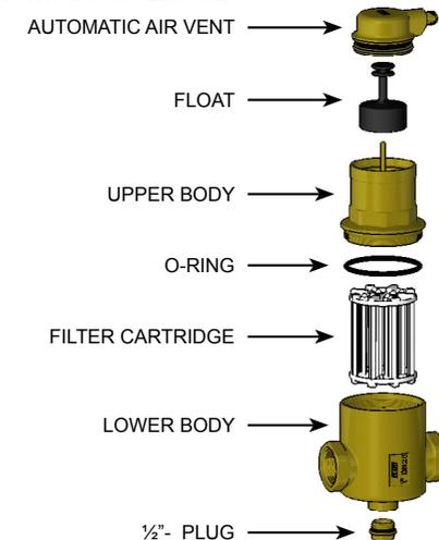
The automatic air vent can be rotated through 360° and purging can be carried out without the need for shut-down.
